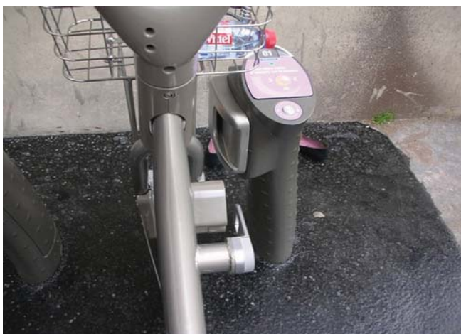
The locking mechanism is attached to the bicycle frame. Image: Richard Ying ( www.flickr.com )
