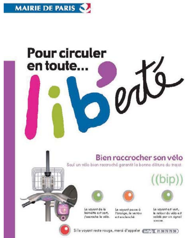
Velib' locking instructions. A green light signifies that the bicycle is available. An orange light indicates that lock is engaging. A green light accompanied by a beep indicates that the bicycle is properly locked. Image: Mairie de Paris
